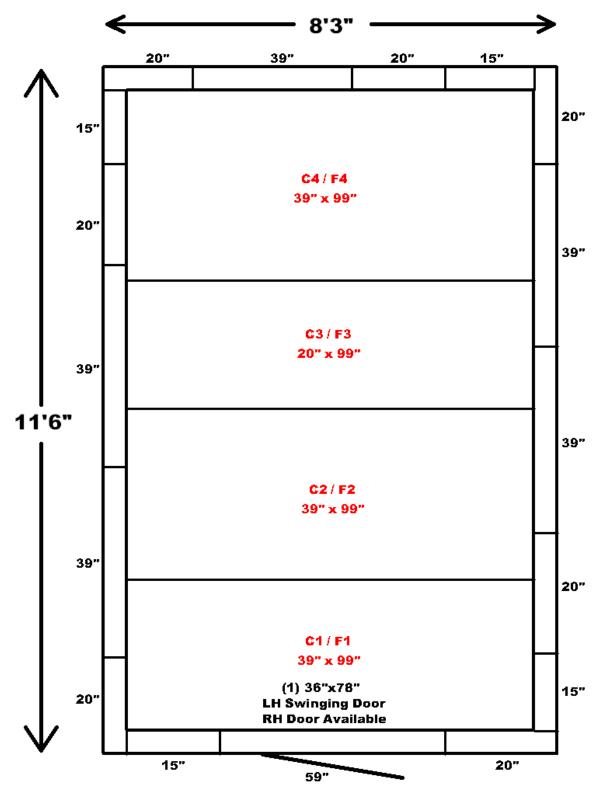
Door can be moved to any wall by swapping door with (1) 20" wall and (1) 39" wall
