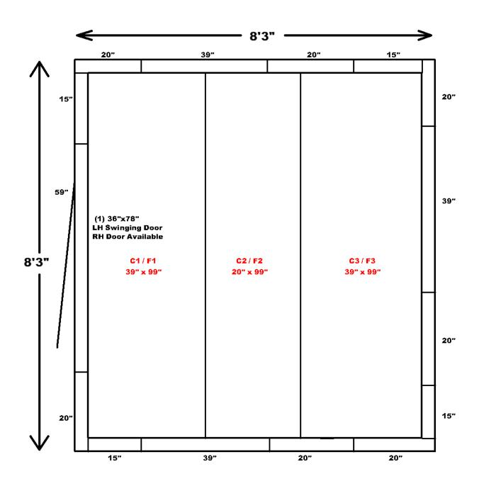
Door can be moved to any wall by swapping door with (1) 20" wall and (1) 39" wall
