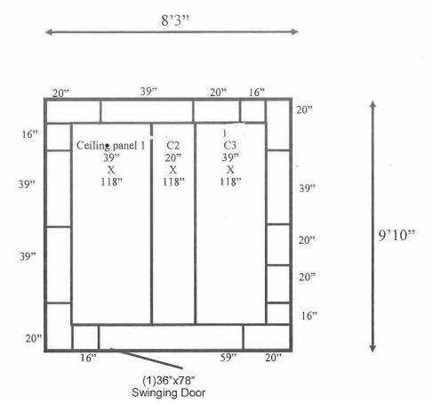
Door can be moved to 9'10" wall by swapping door panel and (1) 20" panel with (1) 39" panel.
