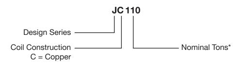
\*At 105°F condensing temperature, 78° wet bulb temperature, 40°F suction temperature, refrigerants R12, R22, R502.
