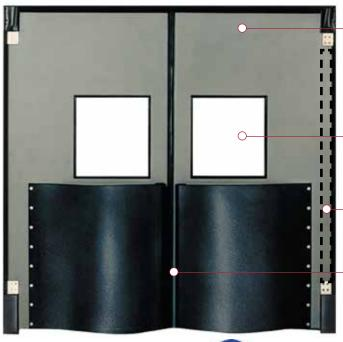
Door Panel - Lightweight, weighing only 3.5 pounds per square foot, is easy to open, operates smoothly and allows for safe passage of personnel and damage free equipment. The overall panel thickness is 1-7/8", the skin thickness is 1/4" thick and the door can be sized up to a 10' x 10'. Rotationally molded polyethylene outer skins retains its properties to -40°F.
