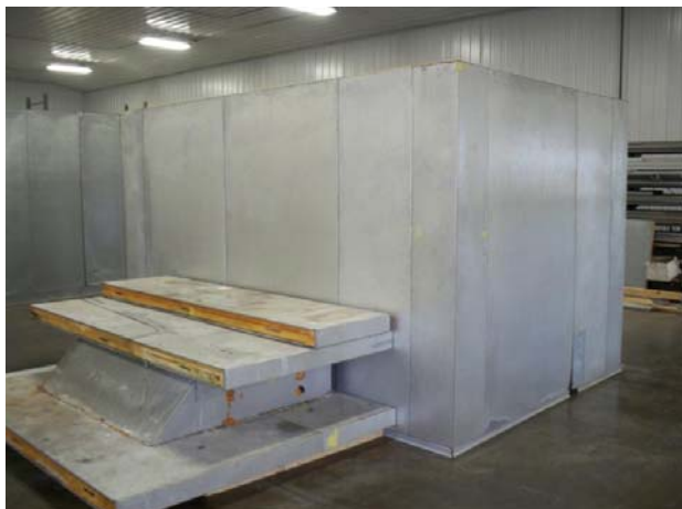
7'9" x 11'7" x 7'4" H (8'6" H with Evap Hood) Walk-In Cooler or Walk-In Freezer
